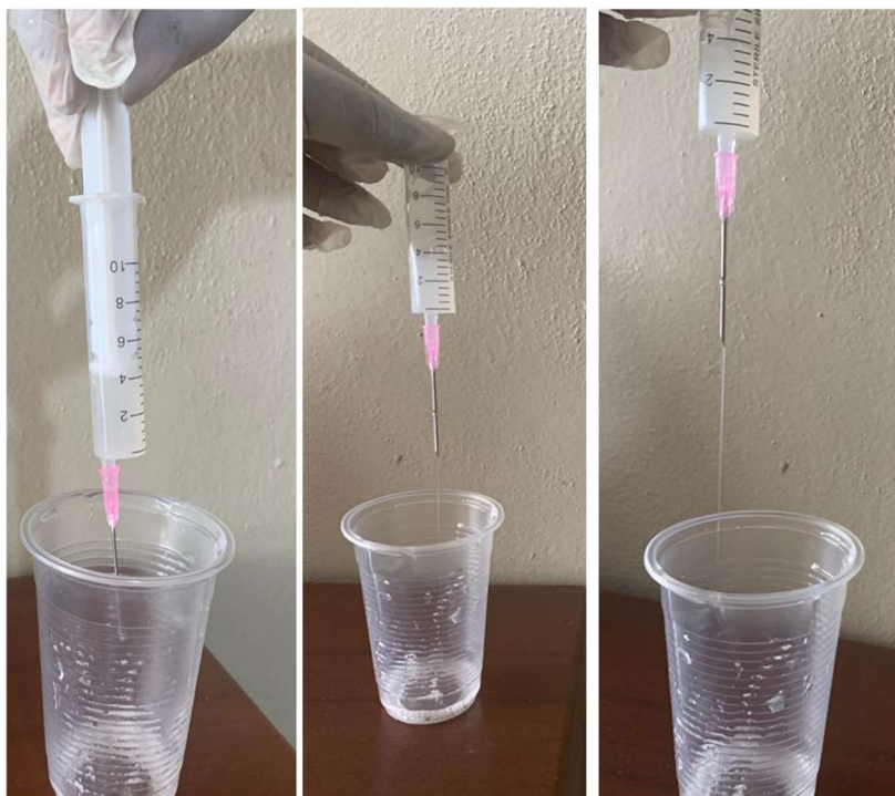
Figure 1: The simple syringe method for measuring relative viscosity of liquid
